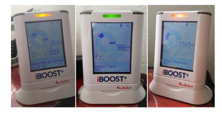
Orange = The hot water is being heated, or electricity being used is coming from the grid and the panels
